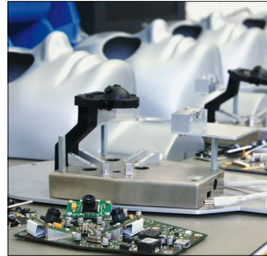
Advanced optical 3D tracking technology for realtime eye surgery simulation
