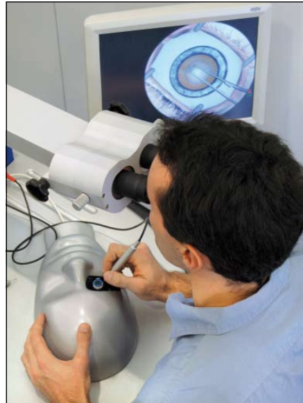
During simulated surgery, the surgeon manipulates realistic handheld instruments which are inserted into an artificial eye
