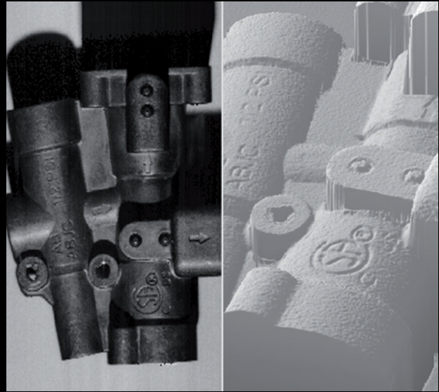
⚡ Resulting intensity image and 3D range map
