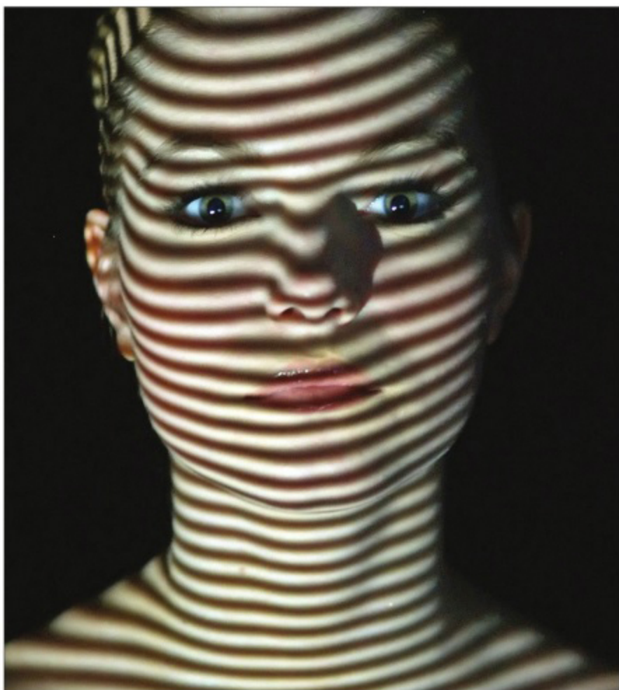
Fringe pattern projection for face capture
