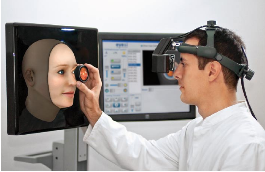
Using a head-mounted display and a model head, physicians can train retinal examination procedures in the same way as with a real ophthalmoscope
