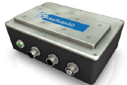
The AreaScan3D features a robust metal housing with IP65 protection, screw-type standard industrial connectors, a 24 V connection, an Ethernet interface as well as hardware and software triggers
