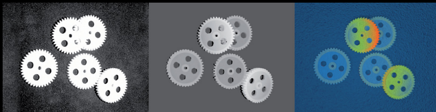
AreaScan3D outputs data directly as a 2D image, gray-scale coded area map, or 3D point cloud.
